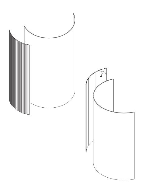
Always make sure the installation surface is clean, even and free of debris. It is best practice to test fit each *Chromaflex* panel on the wall before peeling off the adhesive's protective film from the back. Panels can be installed from left to right or right to left. Regardless of desired installation direction, the exposed tongue on the *Chromaflex* panel must be the leading edge which gets overlapped .5" by the following panel.
